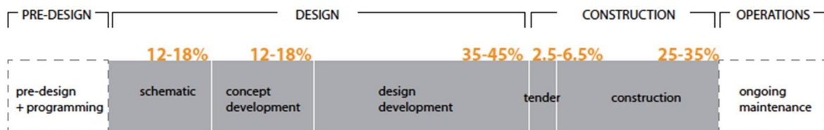
Figure 2.4: Typical architecture design process. Source: Pearl & Oliver, 2013. Based on Canadian Handbook of Practice, 2009. The percentages above the timeline indicate the percentage of time spent on each phase. For instance, 12-18% of the design process is typically spend on schematic design.
