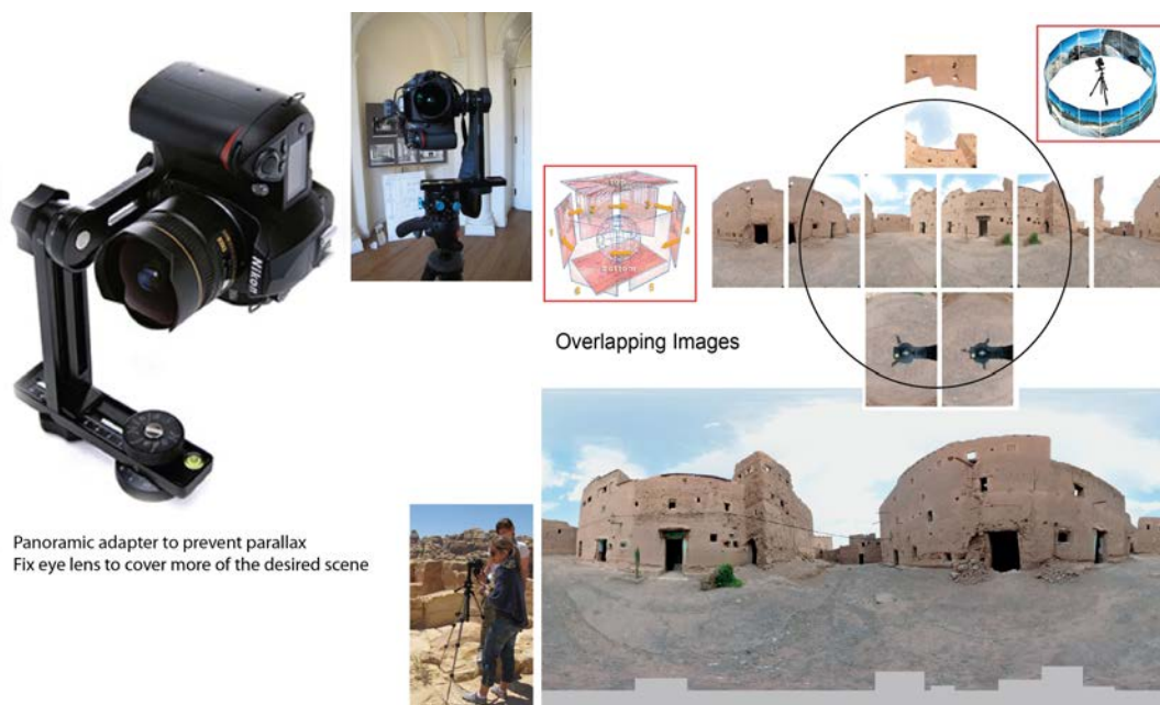
Figure 4 Aspheric panoramic images, prepared by stitching 8 overlapping images of a scene (author).
