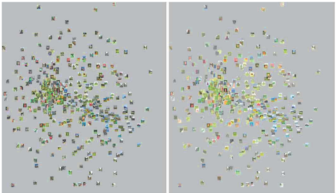
FIGURE II.5 : A MDS visualization map of the Msrc590 based on the VoI distance between segmentations. Left : view map of the (590) color images mapped according to their similarity in term of region-based segmentation result. Right : view map of the segmentation results according to their similarity in the VoI distance sense.
