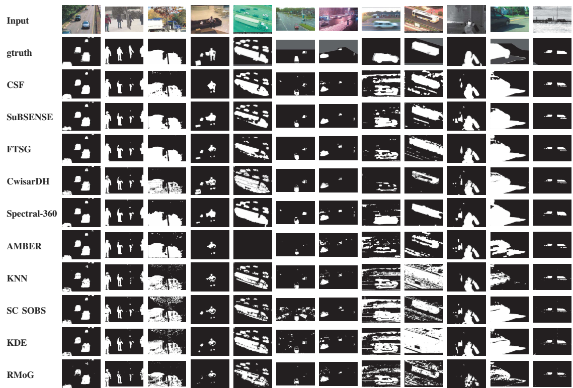
FIGURE 3.5 : Comparisons of results (on different CDnet 2014 images) from different algorithms : from top to bottom respectively ; CSF ( i.e. our [HSV-LAB] supervised fusion approach using the Zivkovitch's BGS), SuBSENSE [9], FTSG [10], CwisarDH [11], Spectral-360 [12], AMBER [13], KNN [2], SC SOBS [14], KDE-ElGammal [15], RMoG [16] algorithm.
