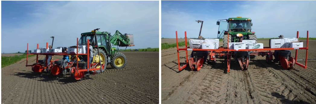
Tractor with modified 3-row cabbage planter, angled view and while planting. The tank of water to gravity feed the suspended wet inoculum can be seen on the fork in front of the tractor (kept mixed with a submerged circulating pump).
