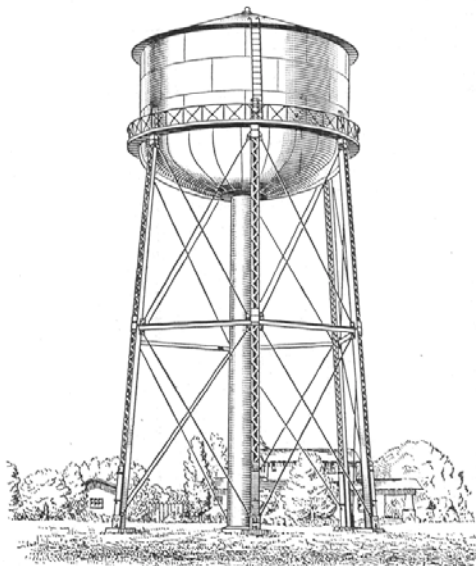
Figure 1.1 Elevated reservoir (steel tank), 1938
