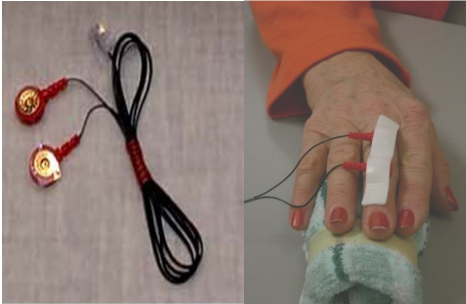
Figure 5. Electrodes and placement of electrodes for use with the Neurometer ®
