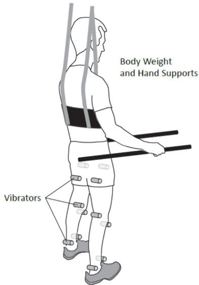
**Figure I. Vibration stimulation device and installation for vibration training**
