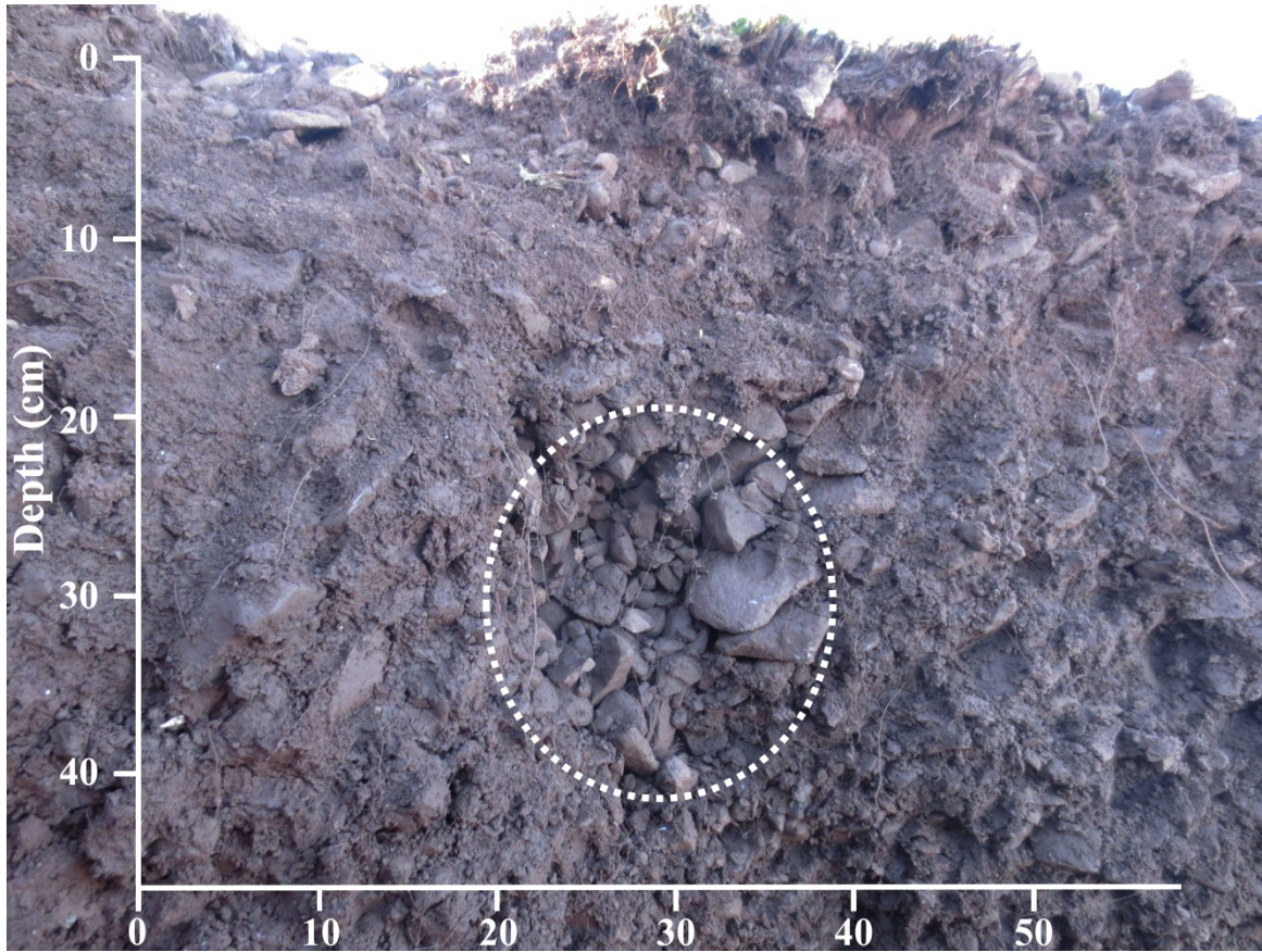
Figure 17. Gravel conduit (15 cm diameter, fines were washed out) in the frontal ridge of the lobe acting as a preferential subsurface flow path.
