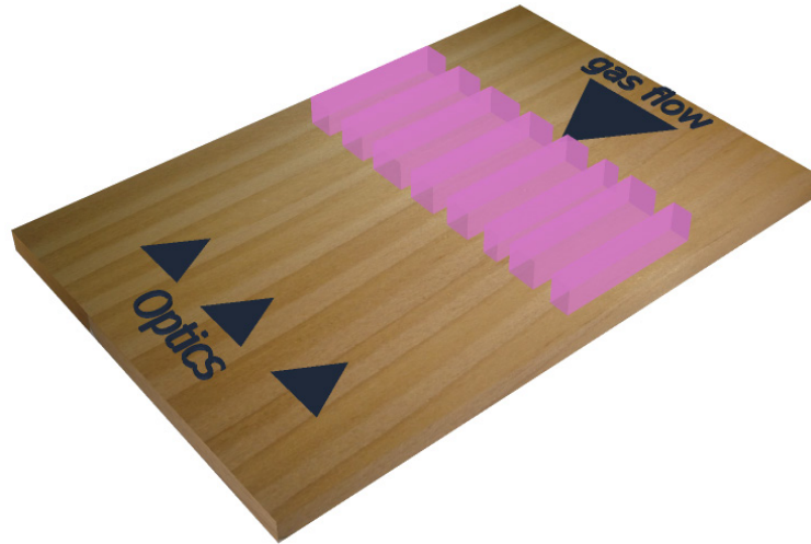
Figure 15 : Position of the optical fibre and digital camera with respect to the plasma emission, wood fiber orientation, and gas flow direction.
