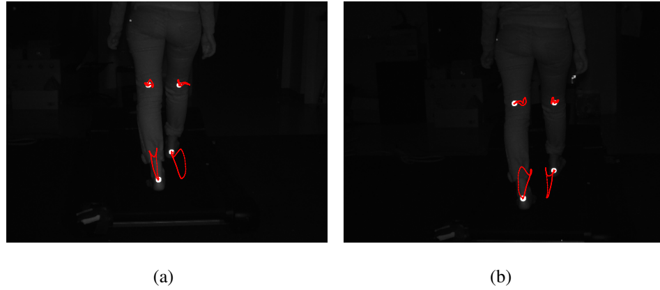
FIGURE 2.13. An example of the tracking of the human gait. An infrared marker is installed on the heel and knee joints of the walking subject. The intensity of the markers is very high so it is easy to isolate it and estimate its centroid subpixel coordinates. Red lines represent the trajectory during one cycle of human gait.
