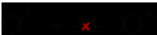
Figure VII.12. Envisioned control experiment with trimethylphenylsilane, which cannot be catalytically transformed into silanol, due to the absence of Si-H bond.
