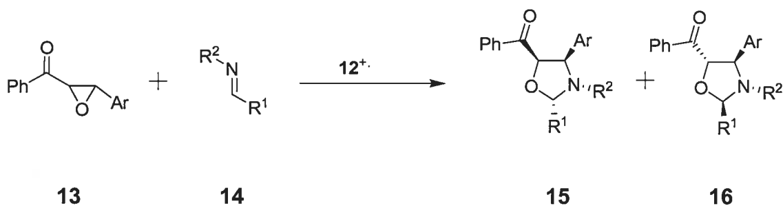
Scheme 2.3 Radical cation-initiated [3+2] cycloaddition of a chalcone epoxide and an aromatic imine. R 1 and R 2 are aromatic groups. 91
