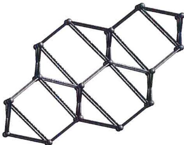
Figure 4.21 Representation of the three-dimensional network formed by the association of tecton 65. The spheres represent the central carbon atom of each molecule, and the solid lines represent the hydrogen-bonding interactions between them.
