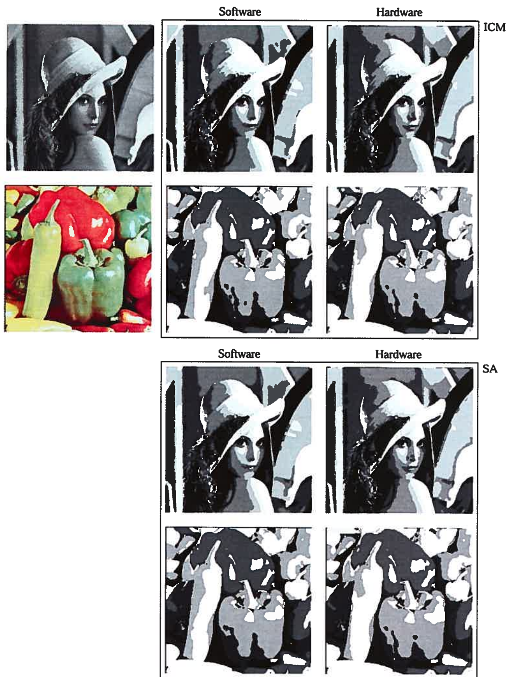
FIG. 4.7 – Gray scale and color image segmented with the software (left column) and hardware (right column) version of ICM (top four images) and SA (four lowest images). In every cases, the Gaussian parameters have been estimated with K-means.
