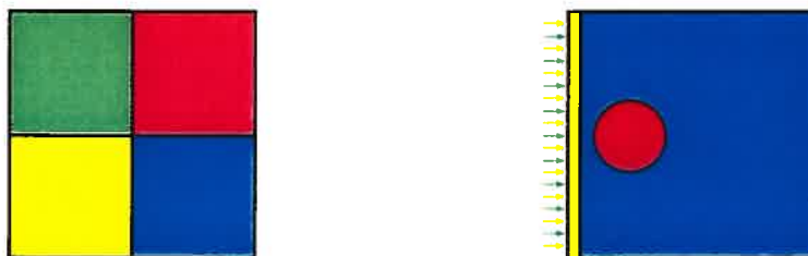
FIG. 5.8. Profile of the initial data for the MHD 2D-Riemann problem (left) and the shock-cloud interaction problem (right)
