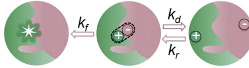
Figure 4.13 – Scheme of the donor-acceptor interface in a bulk heterostructure. k_d : dissociation rate in competition with k_r : recombination rate to form bound polaron pair which can decay with the rate k_f .
