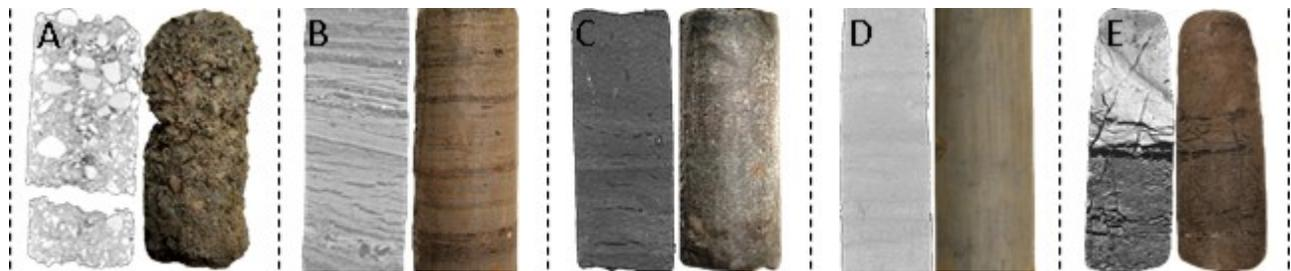
Figure 4. Typical internal structure of permafrost and appearance shown by a tomographic images (left side) and a picture (right side) of each cryostratigraphic unit (A to E). For tomographic images, white indicates dense mineral matter, dark gray indicates ice and mid-tones are proportional to the mixture proportion. The chromatic scale is not fixed and/or absolute but rather individually modulated to increase contrasts and highlight cryostructures.
