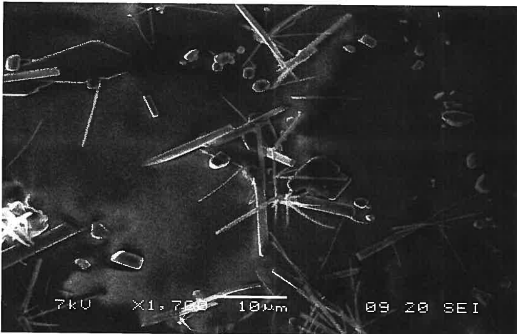
Figure 18: SEM photo of 10% pentoxifylline and 10% DBS film before dissolution showing drug crystals on the film surface.
