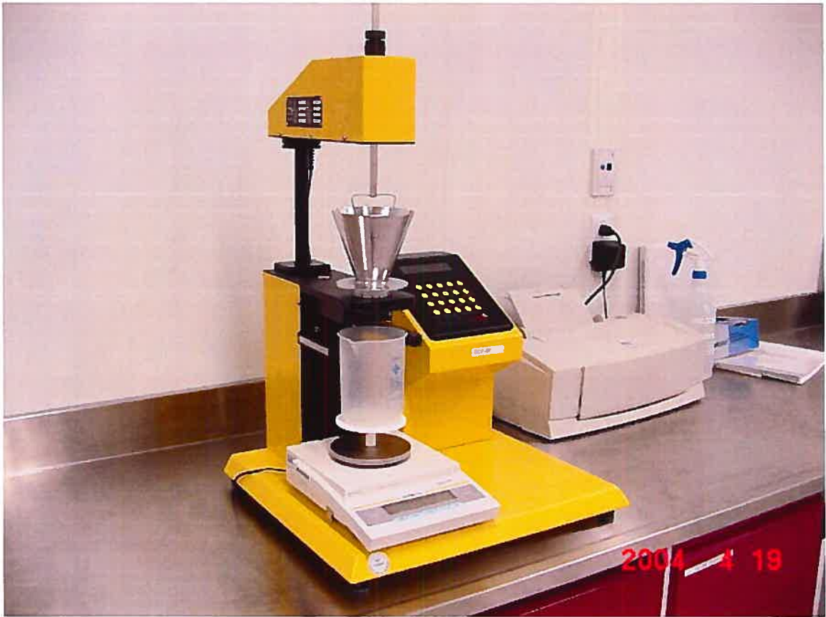
Appendix 1: Pharma test PTG-1 used as a flow meter
