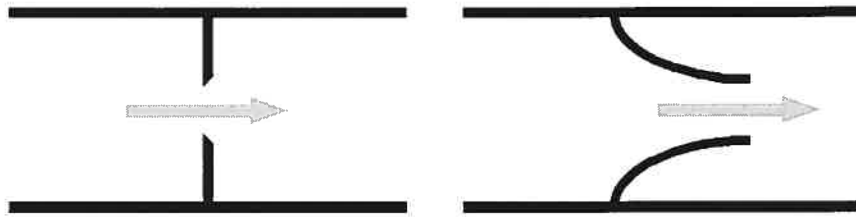
FIG. 8.1 – Schemas of a sharp-edged orifice plate (left) and a funnel-shaped orifice (right).
