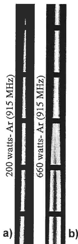
Figure 3-6 : CCD camera recordings of an argon surface-wave discharge at two values of the total absorbed microwave power. Tube radius is 6 mm and field frequency is 915 MHz. The single filament splits into two filaments at higher microwave power level. The longitudinal observation slit made in the cylindrical metallic enclosure is interrupted along a 5 mm length at 30 mm intervals, which accounts for the dark horizontal band in the figure.
