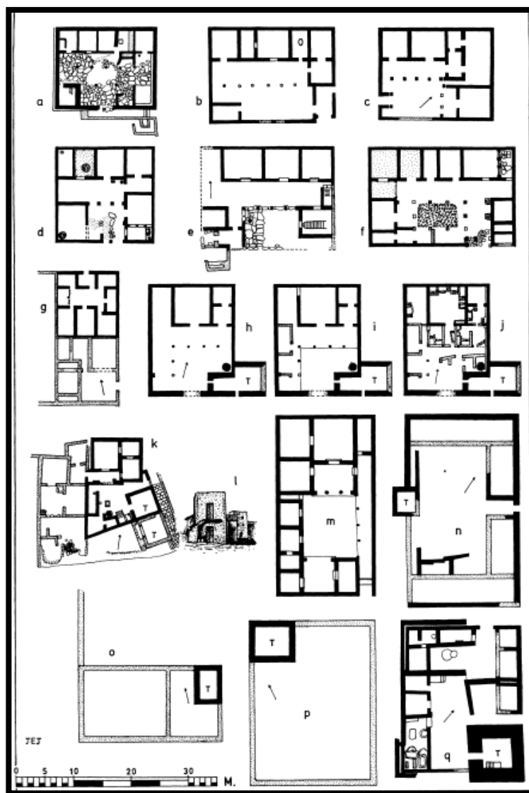
FIG. 16. COMPARATIVE HOUSE PLANS. (a) Vari House; (b) Dema House; (c) Pastar House, Seuthopolis; (d) Olynthus, Villa of the Bronzes; (e) Pastar House, Pella; (f) Olynthus, House Aub; (g) Athens, two houses at north foot of the Areopagus; (h)-(j) Attica, Priest's House at Zoster, original to final form; (k) Colophon, two houses with detached towers and external stairs; (l) tower in Mani with over and under doorways and external stairs; (m) Priene, House 33; (n) Chersonesos, Crimea, farmhouse no. 25, third century B.C.; (o) Thasos, tower-and-court no. 8; (p) Thasos, tower-and-court no. 5; (q) Chersonesos, Crimea, farmhouse no. 26, second century B.C. (T marks towers).
