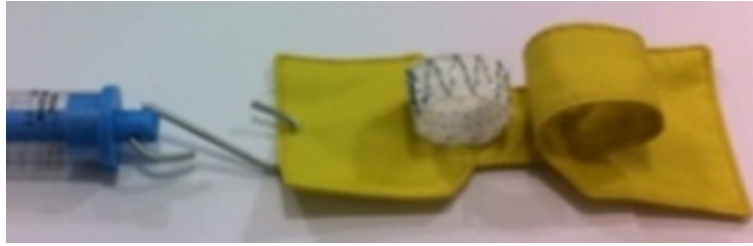
Figure 1.7: Device designed to characterize the radial stiffness of stents.
