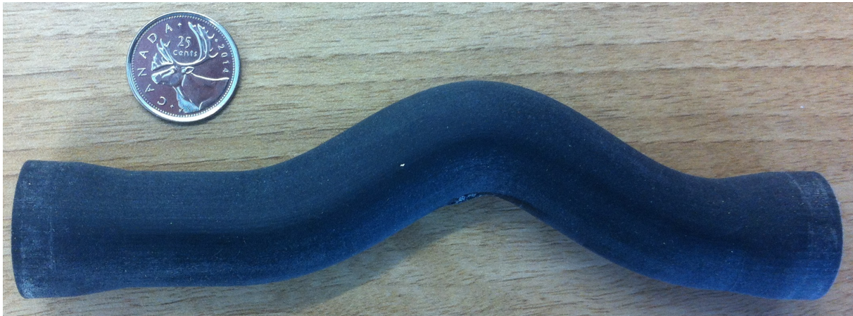
Figure H.1: Simple vascular phantom made of TangoBlackPlus Shore A40 material.
