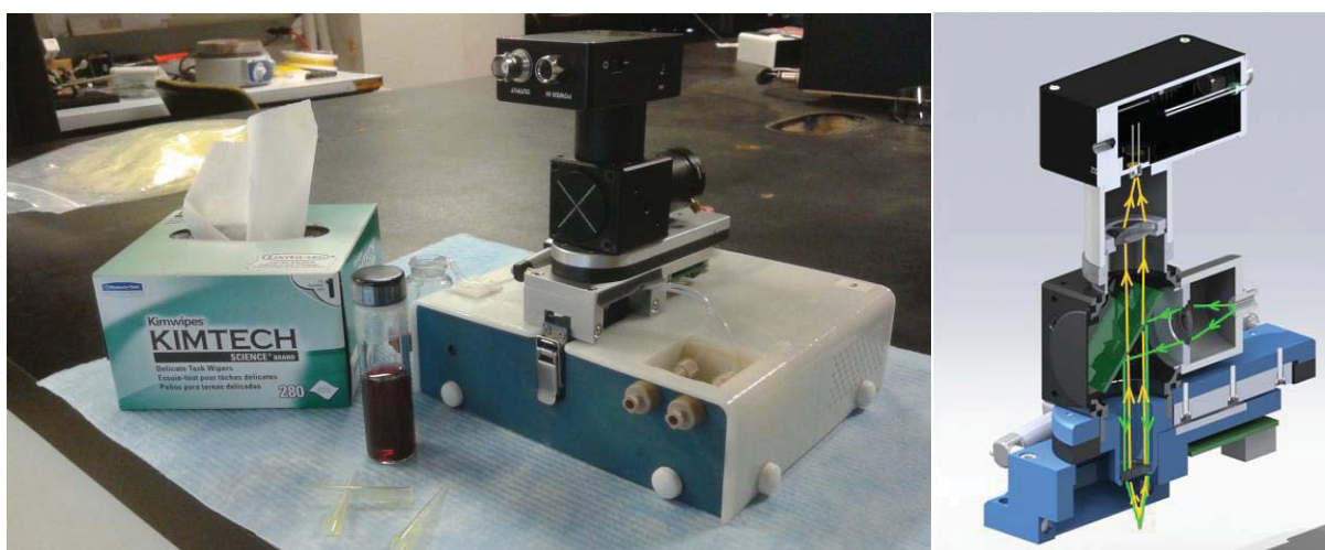
Figure 3.8. SPR instrument with a fluorescence unit. Left) A photograph of the actual unit in the presence of common laboratory items to highlight the small size of the device. The black fluorescence unit was composed of the filter cube (See the white “x”) and the avalanche photodiode at the top of the fluorescence unit. The linear actuator was mounted on the gray aluminum railing and the fluidic cell of the SPR system was underneath the fluorescence unit. Right) Ray tracing of the excitation laser in green and of the emitted light in yellow. Lenses focused the light on the SPR surface and on the avalanche photodiode. The filter cube was composed of a dichroic beam splitter and a long-pass fluorescence filter.
