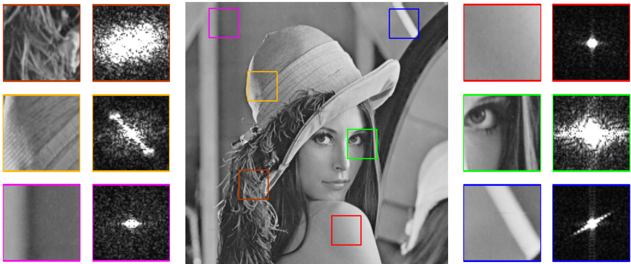
Figure 3.10 – The Fourier transform of a signal captures its frequency variations. Low spatial frequency regions of the image are concentrated around the origin of the Fourier domain while high spatial frequency regions may span the entire Fourier domain. From Belcour [Bel12].
