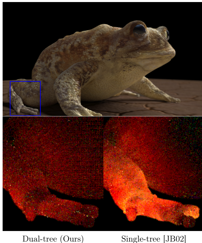
Figure 4.6 – The TOAD scene has a bumpy geometry with detailed textures. We compare the difference images of the multiple scattering term against the ground truth for an equal rendering time (196s). The difference images are scaled by 50 for visualization. Our approach achieves more accurate estimation than the single-tree in the same rendering time.
