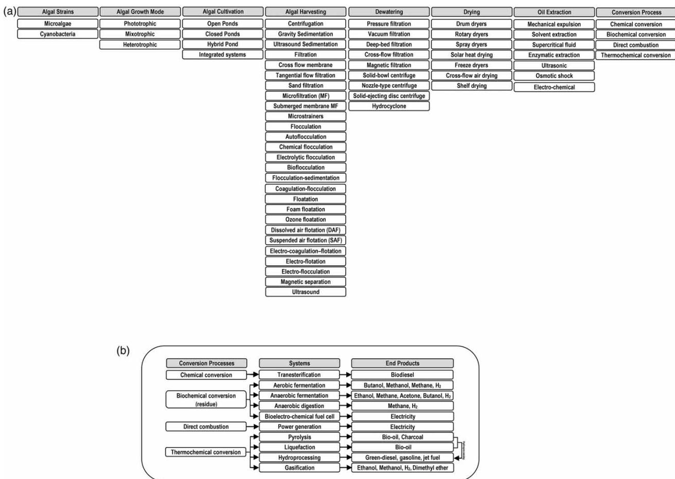
Figure 3. From cultivation to algal biofuel production steps: (a) summary for the steps towards production of algal biofuel and (b) biofuel production via microalgal biomass conversion processes.
