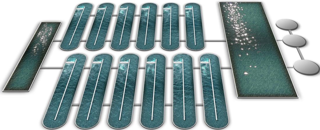
Figure 11: Example of a design of a microalgal cultivation coupled with a domestic wastewater treatment (Leite & P. C. Hallenbeck 2011, *with permission*). Two series of algal ponds in parallel (middle), are fed by the effluent of the wastewater secondary treatment (right). The algal biomass is then settled and harvested in the settling tank (left).
