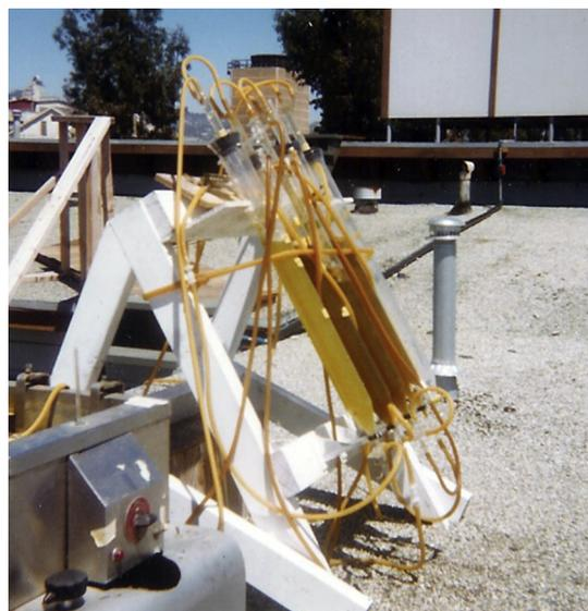
FIGURE 22.3 Tubular photobioreactors operating under “air-lift” conditions were used to demonstrate prolonged (over 30 days) simultaneous oxygen and hydrogen evolution by nitrogen-limited cultures of the heterocystous cyanobacterium, *Anabaena cylindrica*. Source: Miyamoto et al 1979d. (For color version of this figure, the reader is referred to the online version of this book.)
