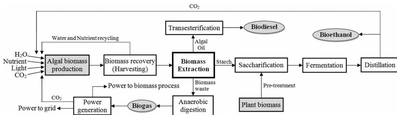
Figure 1. Integrated system for biodiesel, bioethanol, biogas, and power generation.
