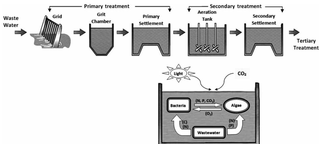
Figure 1. Contrast between conventional wastewater treatment and wastewater treatment using algal ponds.
