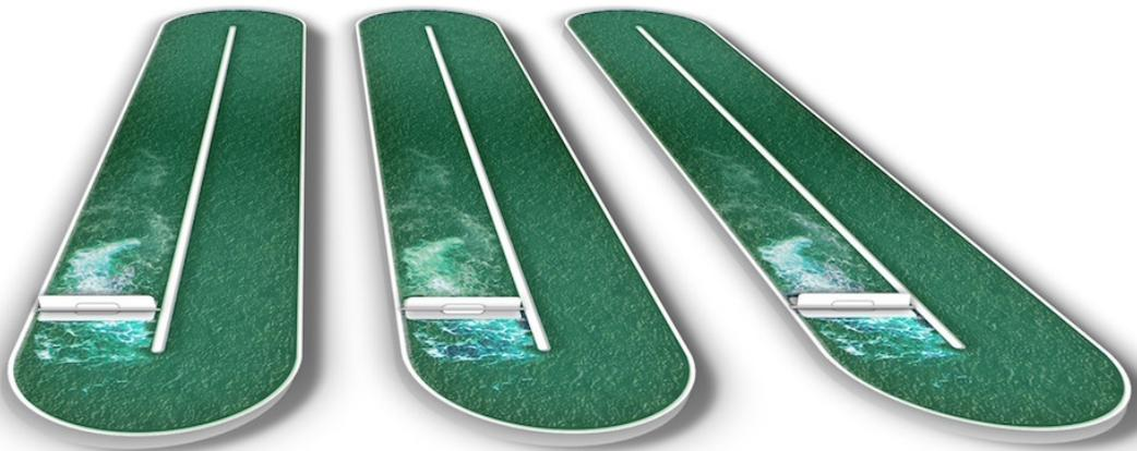
Figure 9: Design of a raceway open pond. (Image credit: Ivan Castilho/CC-BY-SA-3.0)
