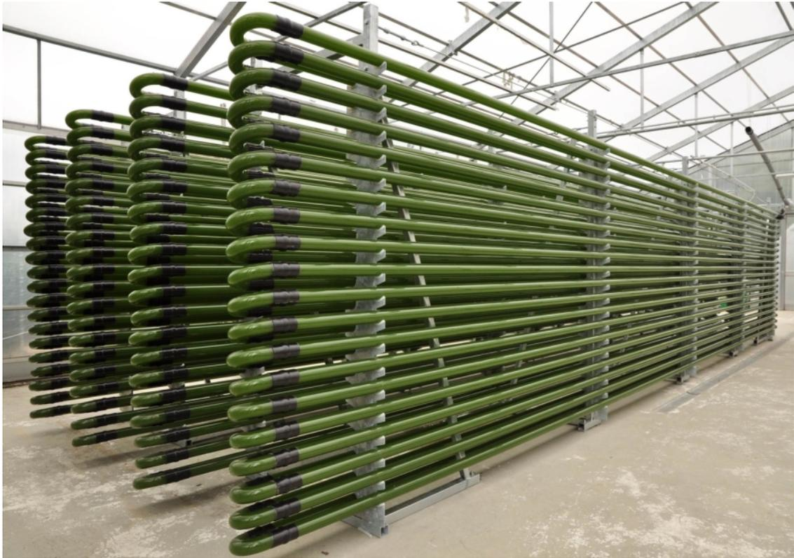
Figure 8: Horizontal tubular photobioreactor of 4000 liters capacity. (*Photo credit: IGV Biotech/CC-BY-SA-3.0*)
