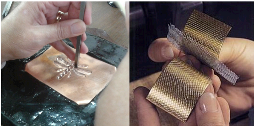
Figures 10 and 11: Examples of cold connections, chasing (left) and texturing metal (right).
