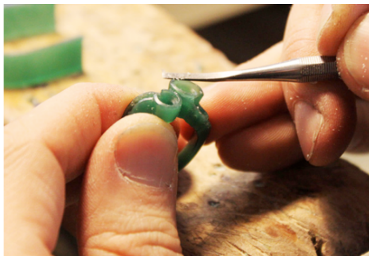
Figure 14: Hand Carved Wax for a Multiple Marquis Cut Diamonds Band Ring. From diamondgalleriesd.com
