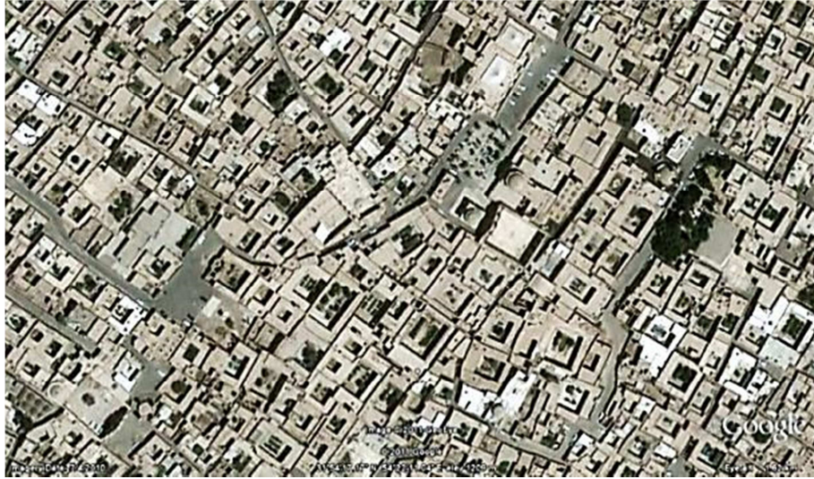
Figure 2-11: The northern-southern orientation of courtyards, Kashan historic center, Iran. The figure shows that courtyards have followed mostly the same orientation in a specific region. Retrieved from www.maps.google.com
