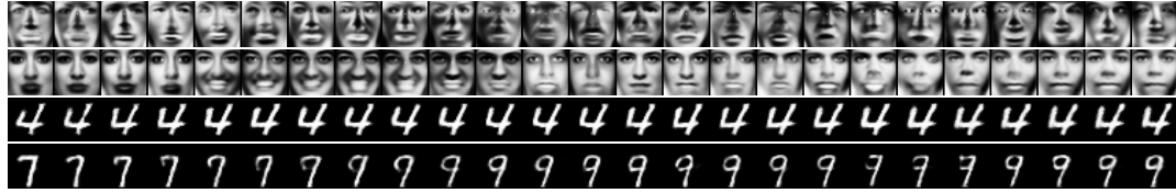
Figure 8.2 – Sequences of 25 samples generated with a CAE on TFD (rows 1 and 2, respectively for 1 or 2 hidden layers) and with an RBM on MNIST (rows 3 and 4, respectively for 1 or 2 hidden layers). On TFD, the second layer clearly allows to get quickly from woman samples (left) to man samples (right) passing by various facial expressions whereas the single hidden layer model shows poor samples. Bottom rows: On MNIST, the single-layer model gets stuck near the same mode while the second layer allows to mix among classes.
