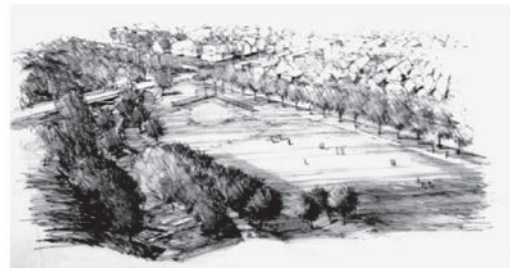
Large parks and school grounds are integral components of the site's ecological infrastructure. They provide on-site bioremediation and infiltration for large storms, and they become shallow retention basins during 20 to 100 year storm events.
