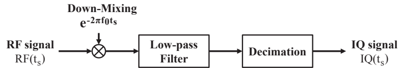
Figure 4.7: Conversion of a radio-frequency (RF) signal, acquired with respect to the sample time t_s , to in-phase quadrature (IQ) data. Modified from [30].
