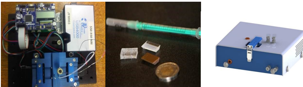
Figure 6.2 (Left) Picture of the inside of the prototype system. Its dimensions: 181(L) x 166 (w) x 55 (H) mm. Its weight: 1.3kg. (Middle) Picture of gold-film coated disposable prism and disposable PDMS fluidic cell next to a dime. (Right) Graphical depiction of the casing of the SPR system.
