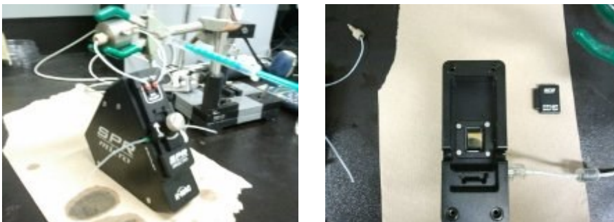
Figure 6.8 Picture of left) the KMAC SPR micro system. Dimensions: 45(w) x 140(L) x 130(H) mm and right) sensor chip deposition before microfluidic cell mounting on KMAC SPR micro.
