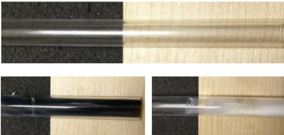
**Figure 9:** Optical images of the discharge tube (top) before plasma deposition (pure argon gas), (bottom left) following treatment in Ar/HMDSO plasmas, and (bottom right) after treatment in Ar/HMDSO/O<sub>2</sub> plasmas. A wood sample was placed in the background for clarity.
