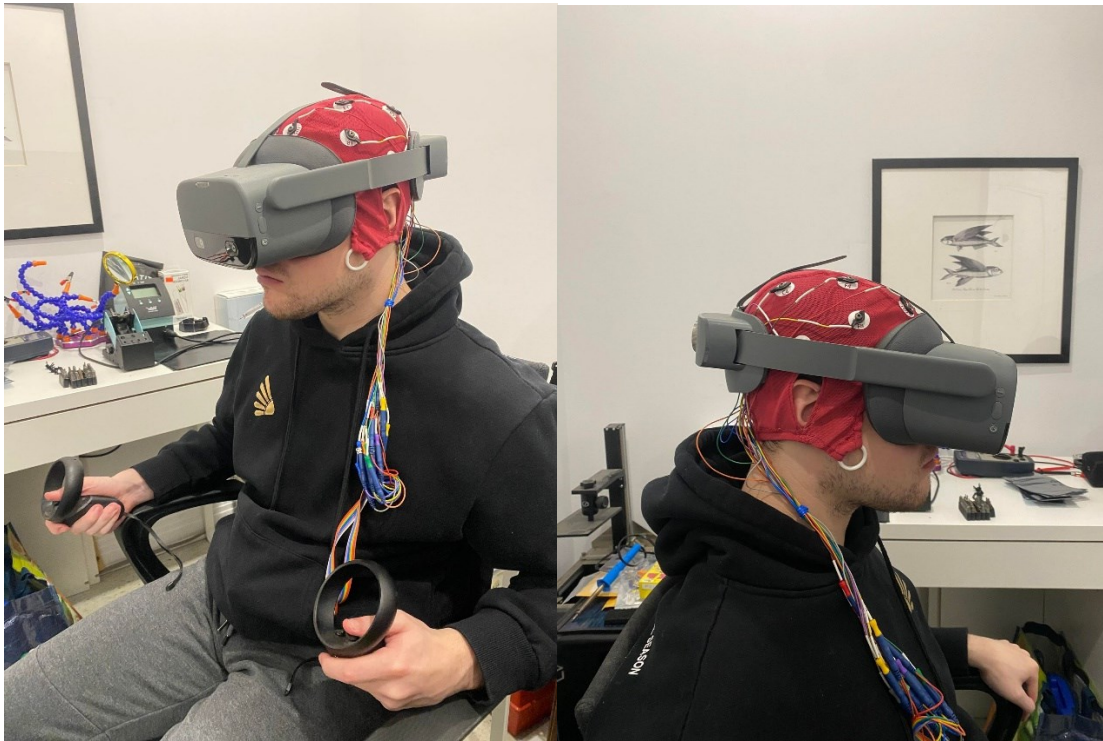
Figure 2 Apparatus of the Emotiv Epoc EEG headset with control remote and VR headsets
