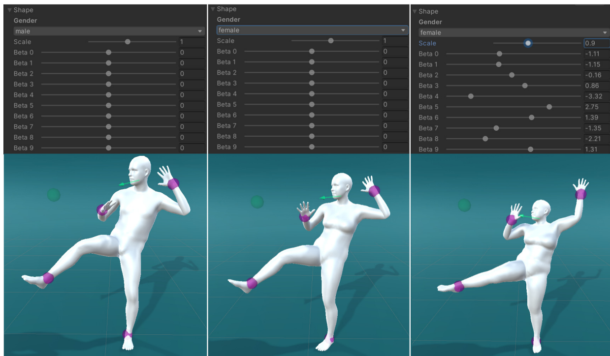
Fig. 5.4. Morphology-aware learned IK. Left: posing the average male SMPL character. Center: result of modifying only the SMPL gender parameter. Right: result of additionally modifying the SMPL \beta shape parameters.
