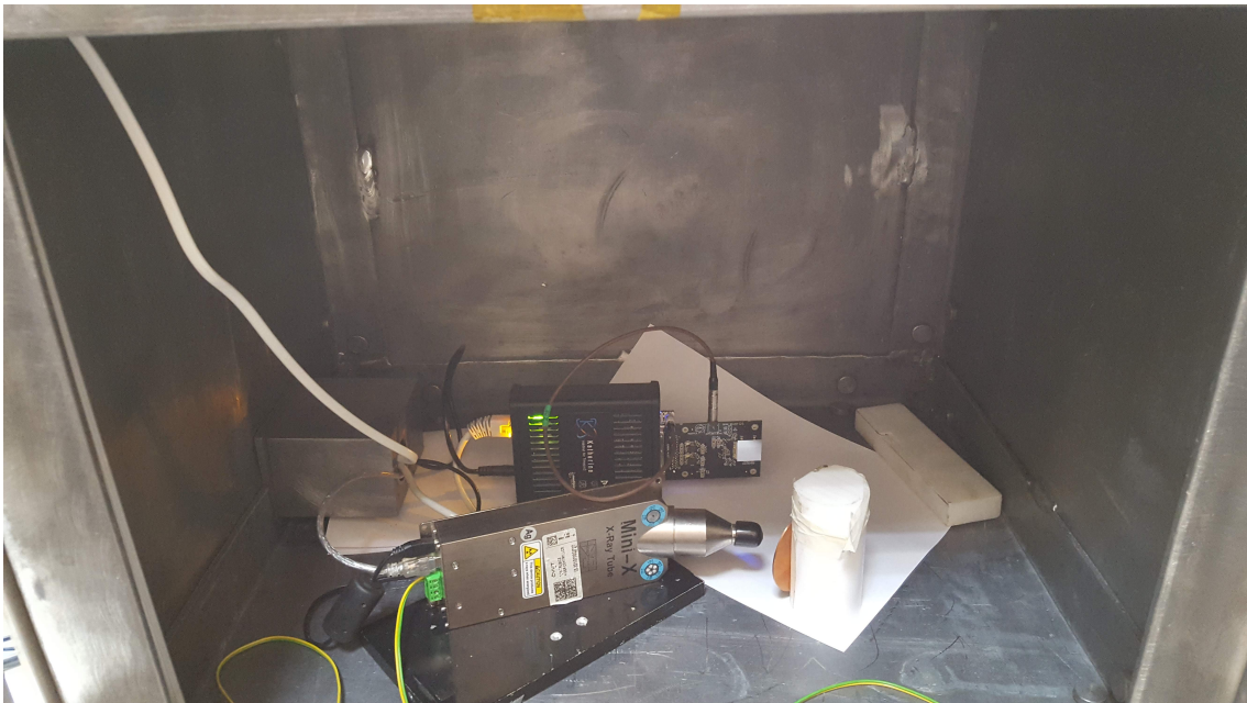
Fig. 5.2.2. The TPX3-Si, connected with a Katherine interface[50], in the calibration setup. The detector, fluorescence sample (Cu is shown), and Amptek Mini-X tube are housed in a radiation-hermetic lead lined box. The calibration is performed at the IEAP in Prague.
