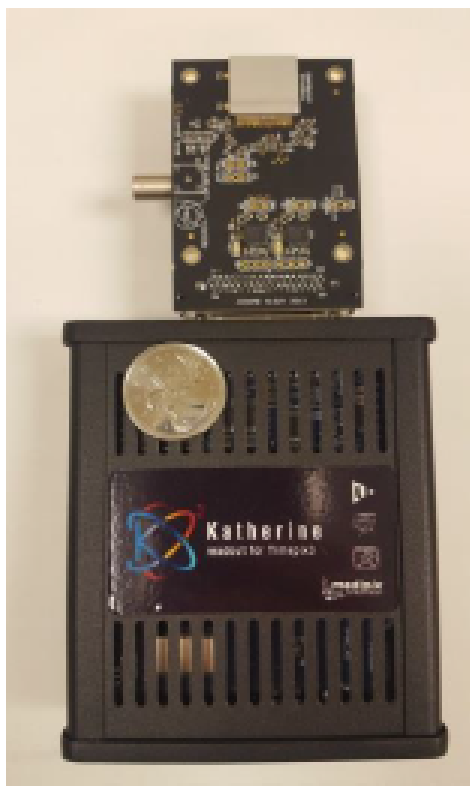
Fig. 1.4.1. A Timepix3 detector equipped with a Katherine readout system interface.
