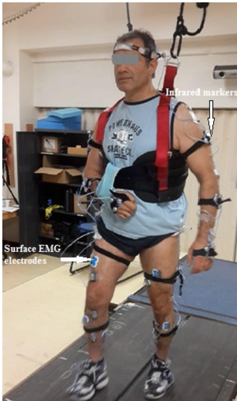
**Figure 4.4.** After the installation of infrared markers, participants walked on an instrumented split-belt treadmill. The treadmill was used to apply unpredictable gait perturbations by increasing or decreasing the speed of one of its belts.
