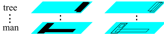
Fig. 6.4. Blue indicates 0 and black indicates 1. (Left) The per-class mask constructed from the layout by many previous methods makes it impossible to distinguish unique object instances in several cases. (Right) Our mask consists of instance boundaries making it easier for the model to distinguish unique object instances using no extra information than already contained in the layout.
