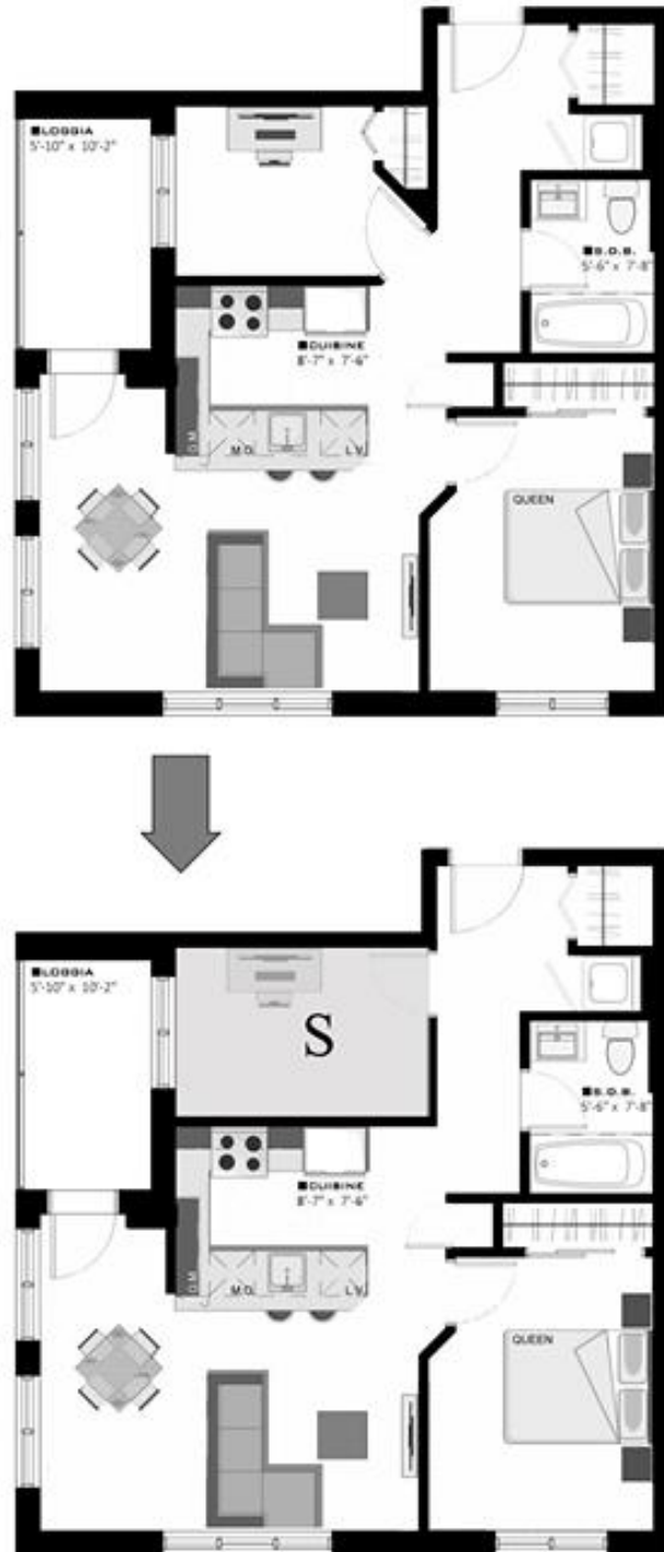
Figure 5.23. MUZ condominium project, Montréal. Floor plan with the implementation of “supplementary space” (“MUZ condominium”, 2013)
