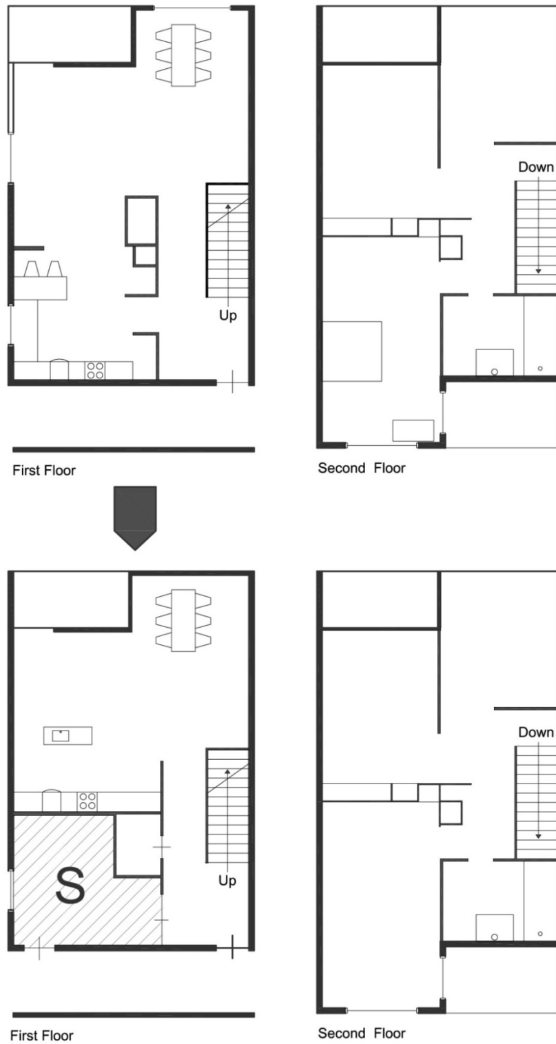
Figure 5.24. Top: Maisonette floor plan, Bennett project, London, 1971 (Sting, 1975), Bottom: Implementation of supplementary space
