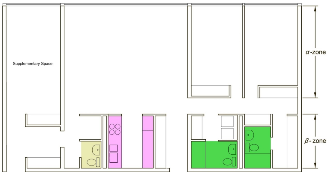
Figure 6.36. Integration of services pods in the " \beta " zone of the longitudinal generic model
