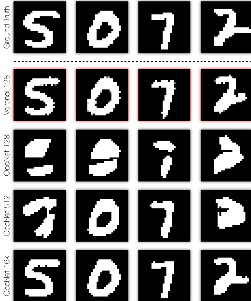
Fig. 4.6. Qualitative results of our autoencoding approach on the MNIST dataset. Compared to OccNet, we are able to achieve comparable accuracy with representations containing two orders of magnitude less parameters (128 vs 16k).
