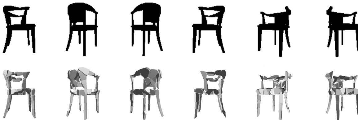
Fig. 4.10. 360 degree visualization of a learned chair represented using our Voronoi-based representation. The top row shows the ground truth silhouette while the bottom row shows the final learned 3D model for the same poses.
