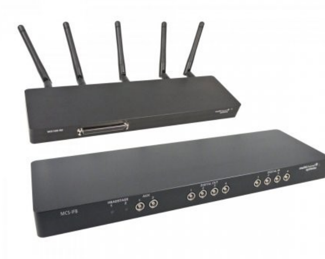
Figure 12. – Representative image of A) the wireless data acquisition system (Multichannel W2100 System) and B) the headstage used for the electrophysiological stimulations and recordings in the uncoated electrode in vivo experiment.
