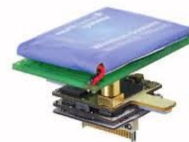
Figure 12. – Representative image of A) the wireless data acquisition system (Multichannel W2100 System) and B) the headstage used for the electrophysiological stimulations and recordings in the uncoated electrode in vivo experiment.
