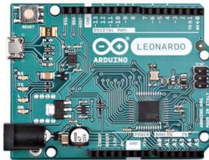
Fig. 2.3. The Arduino Leonardo microcontroller board 5
