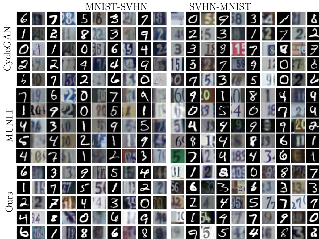
Figure 3.2. Qualitative comparison of CycleGAN and MUNIT with our methods on MNIST to SVHN. For each figure, the even column c correspond to the source samples and the odd column c + 1 correspond to source samples translated to the target domain. The first row of figures are the results obtained on CycleGAN. The second row of figures are the results obtained on MUNIT. The last row of results are the results obtained using our approach.
