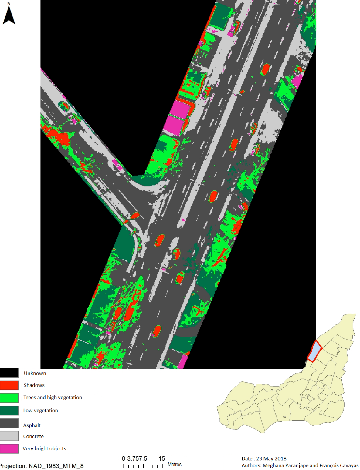
Figure 21 Urban surface materials of a portion of Montreal North using K-means clustering with RGBI 20cm ortho-images
