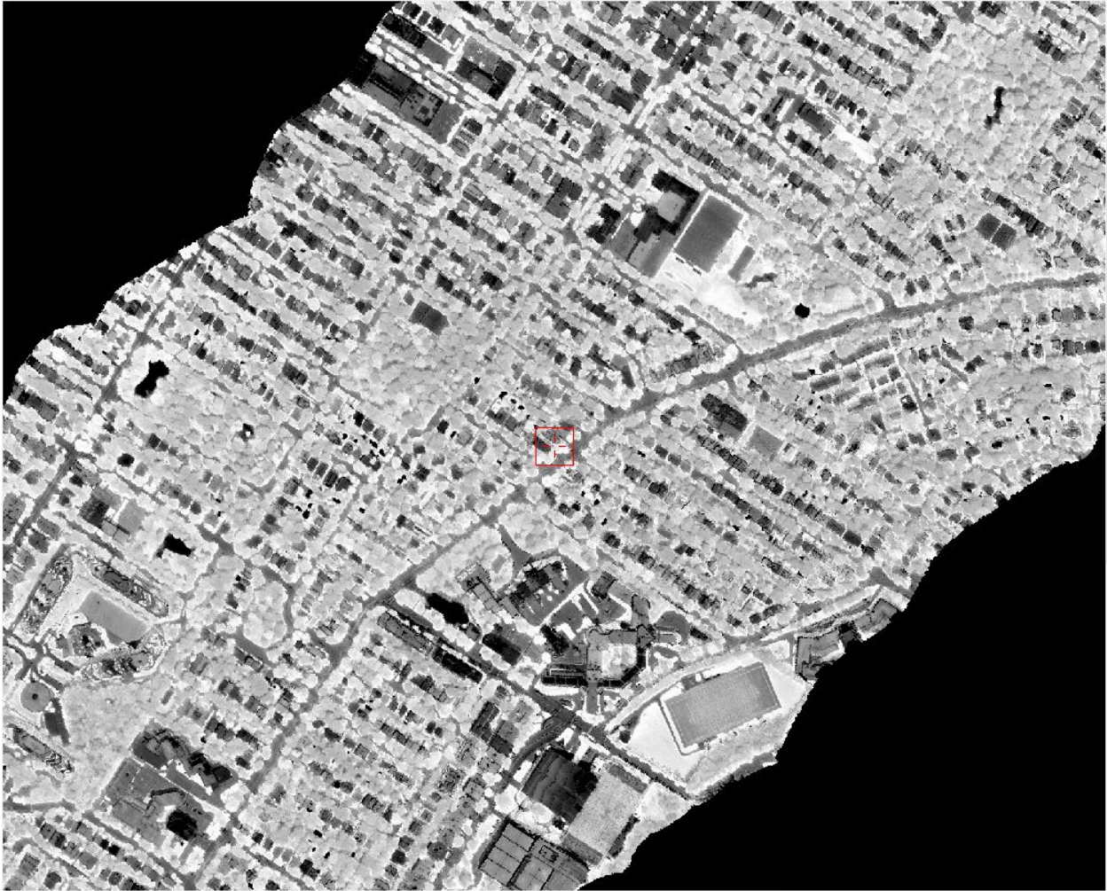
Figure 33 Example of output image after running the shape similarity metric testing for a reference spectral signature representing grass from ASD spectral library (light shades of grey indicate pixels that are more likely to resemble grass, while darker shades are less likely to resemble grass)
