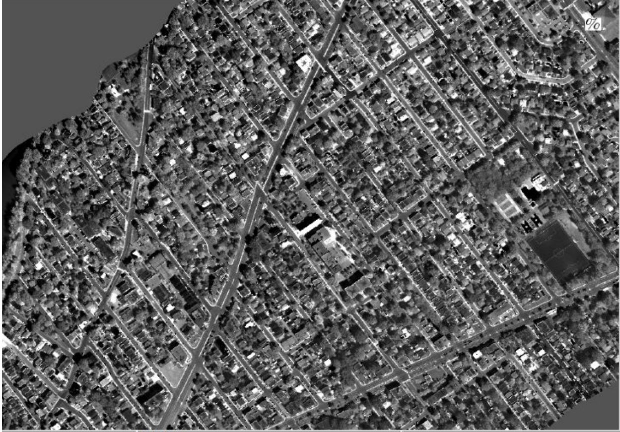
Figure 15 Linear spectral unmixing results using hyperspectral CASI 1500 imagery of Montreal North (Montreal, Qc, Canada), bright shades represent higher proportions of concrete, while dark shades represent lower portions of concrete
