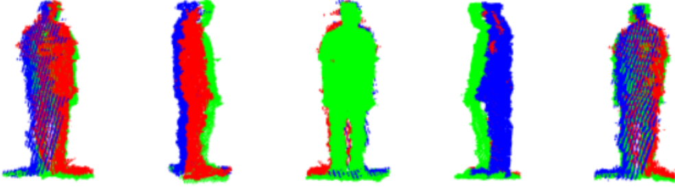
FIGURE 3.6: Reconstructed point clouds of a human body with the same posture. This process was done by applying the proposed Algorithm 1 on noisy depth information. The points corresponding to ground can be easily removed as a post-processing step based on the ground calibration.
