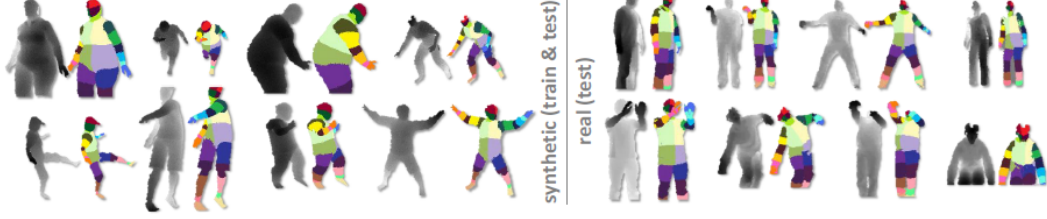
FIGURE 2.19: Synthetic and real data for training the random forest integrated into the Kinect [132]. Each pair of images consists of a depth image and ground truth labeled body parts.
