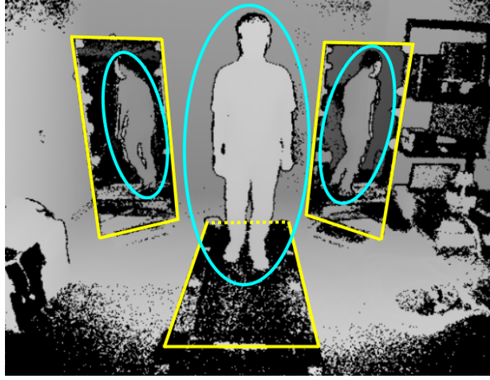
FIGURE 5.3: A depth map captured by our system, in which there are 3 collections of subject’s pixels (highlighted by cyan ellipses). The two mirrors and the treadmill are highlighted with yellow rectangles.
