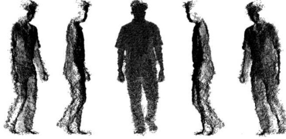
FIGURE 6.2: The point cloud reconstructed from a depth map using the method [107].
