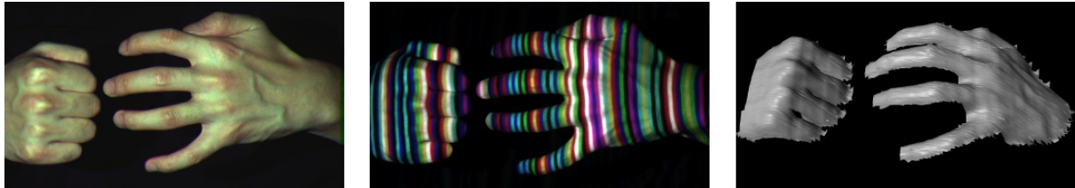
FIGURE 2.10: Reconstructing the shape of two hands in the study [165]. From left to right: real scene with two hands in front of a dark background, the scene under illumination with color-striped pattern designed based on the Bruijn code, reconstructed model shown at a different viewpoint.
