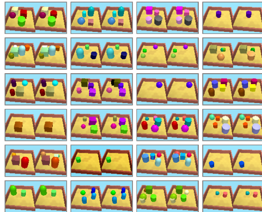
FIGURE 6.8. 3D scene reconstructions. The SPIRAL agent is trained to reconstruct 3D scenes by emitting sequences of commands for the MuJoCo environment. In each pair, the left image corresponds to the model’s output while the right one is the target. Our method is capable of accurately inferring the number of objects, their locations, sizes and colors.
