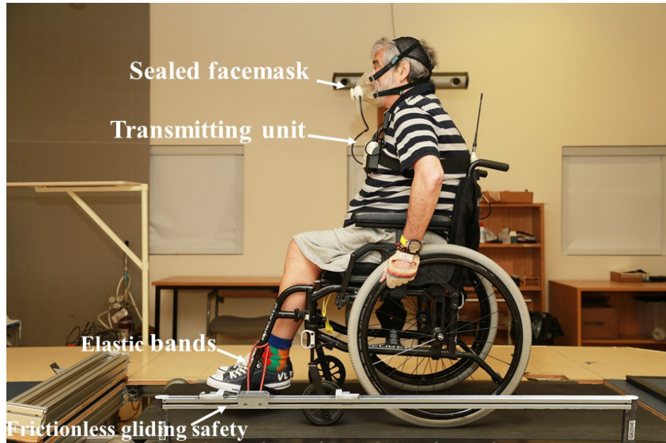
Figure 5.6 Experimental set-up when performing the WPT Treadmill .
