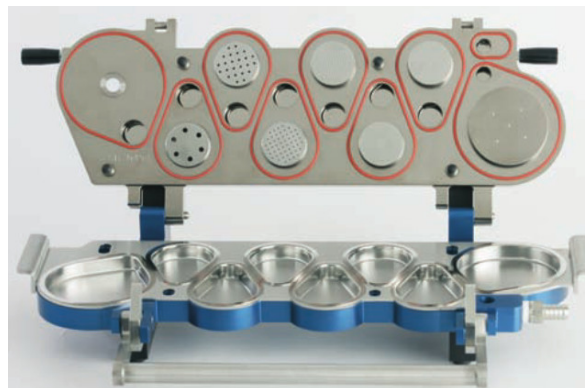
Figure 29: New generation cascade impactor. Taken with permission from Copley Scientific.
