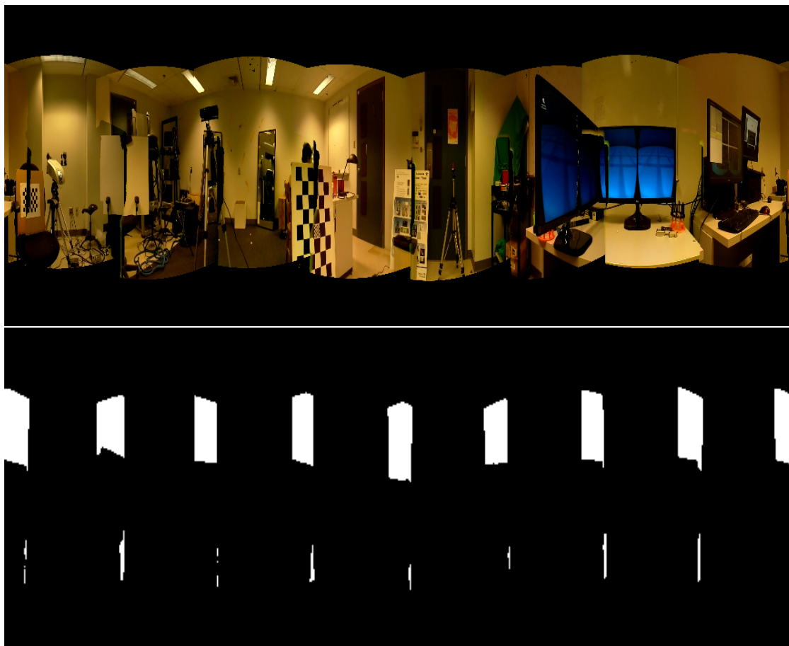
Figure 3.9 – Sample tangential panorama (top) with mask (bottom) illustrating overlapping pixels (seen by two cameras). Smaller overlap is caused by camera occlusion.
