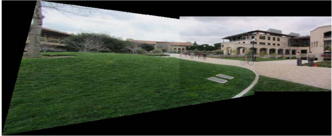
Figure 1.2 – Sample of two stitched images with a camera. The center of camera is fixed and only rotate camera to capture second image
