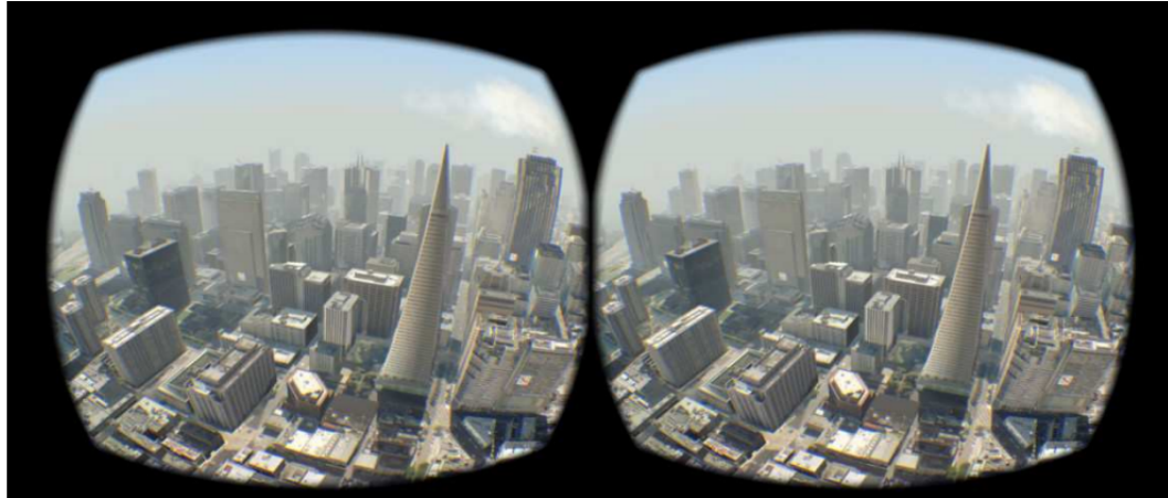
Figure 1.1 – Left and right eye views are created inside the headset, while also taking into account the user’s looking direction.
