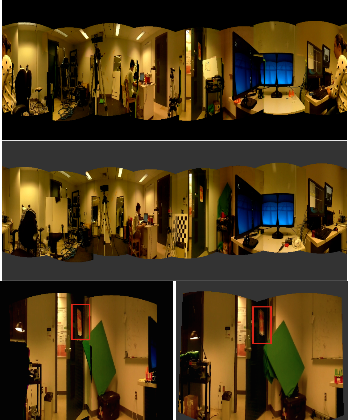
Figure 3.13 – Sample panoramas with tangential model (top) and radial model (middle). At bottom, a single object highlighted with a red rectangle illustrates the difference between tangential model (left) and radial model (right).
